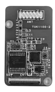
Power 17mA Dimension 35 x 25 x 5mm You can get signal strength easily like above 2 items. Frequency: kHz,MHz,GHz Band Applicable to custom order
